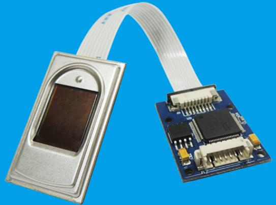
CAMA-AFM288 is an ideal OEM capacitive fingerprint Sensor Module which combined CAMABIO fingerprint algorithm and FPC1011 fingerprint sensor. And it also equipped with microcontroller chip and flash memory. With its' compact size, it can be easily integrated into different biometric recognition devices like time attendance, access control, smart door lock, etc.
