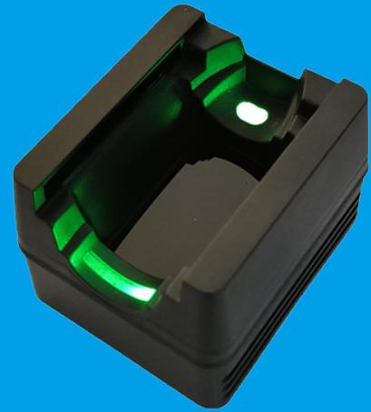
CAMA-FVM2201 is an OEM finger vein module developed by CAMA Biometrics. It integrated optical sensor,MCU,finger vein recognition algorithm,flash memory all together. It can suit for variety of embedded and online authentication mangement applications.
